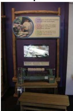
I can put my feet on the pedal to make the wood spin. There is a tool made of wood and metal. I can hold the tool gently against the spinning wood.
